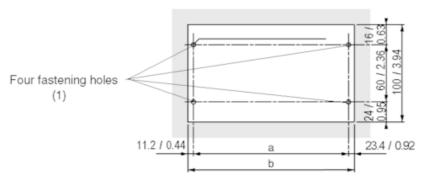
(1) The diameter of the fastening holes must allow use of M4, M5, M6 and UNC #6 screws.
